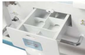
The humidity reservoir is removable
